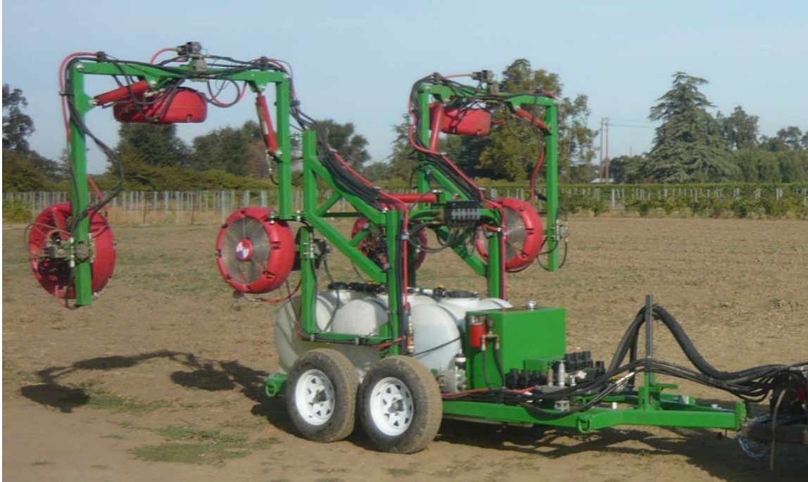
Multi-row sprayer showing spray tanks and trailer details. Photo credit: R. Billing
