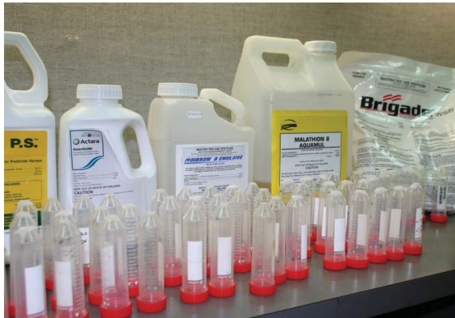
Figure 1. Centrifuge tubes were used for determination of Lygus bug susceptibility to commonly used insecticides and their tank mixes.
