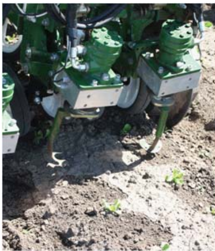
Photos 4 & 5. The Tillet Weeder is a commercially available mechanical weed control machine that uses computer technology and a spinning blade to remove weeds. On left: The disc-shaped cultivation blades are lifted up so you can observe the notched cut-out that allows the blade to spin around crop plants. On the right: Thinning lettuce.
