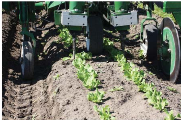
Photos 4 & 5. The Tillet Weeder is a commercially available mechanical weed control machine that uses computer technology and a spinning blade to remove weeds. On left: The disc-shaped cultivation blades are lifted up so you can observe the notched cut-out that allows the blade to spin around crop plants. On the right: Thinning lettuce.
