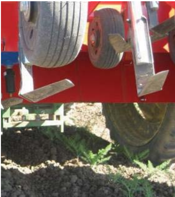
Photo 3. Knives in the open position
